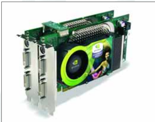
nVidia's SLI technology allows two cards to be connected in parallel
