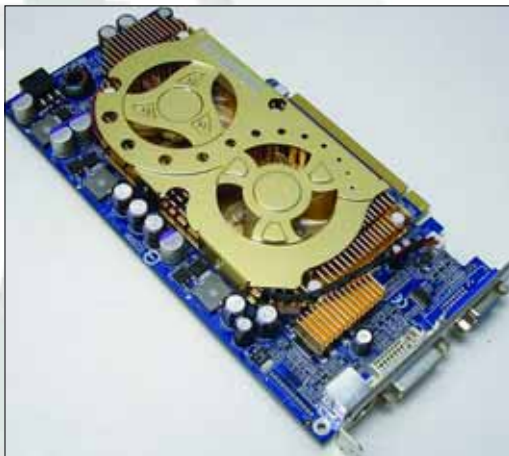
Card makers have started putting two GPUs on cards to get the best performance possible. It gets better when you use two of these dual-GPU cards in SLI or CrossFire mode
