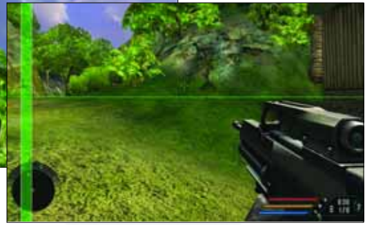
Split-frame rendering, as seen in FarCry . The horizontal green line distinguishes between the rendering done by each card
